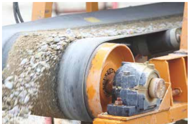
SIT-LOCK® 1 used for a conveyor belt pulley.
