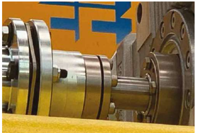
SIT-LOCK® 3 used for a disc coupling.
