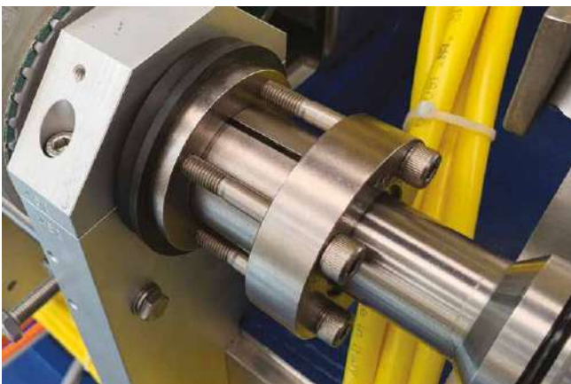
Locking two shafts using SIT-LOCK® 10, nickel-plated version.
