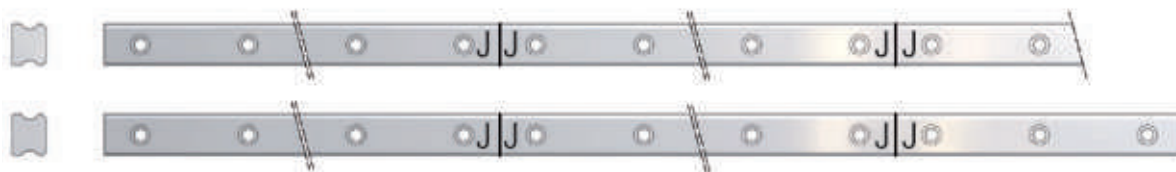
Figure 3.6 Marking of jointed rails
