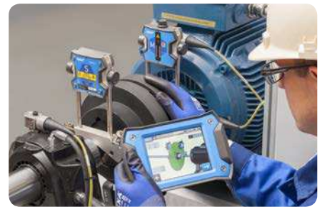
The TKSA 31 communicates via USB cables, but it has the same alignment performance as the TKSA 41.
