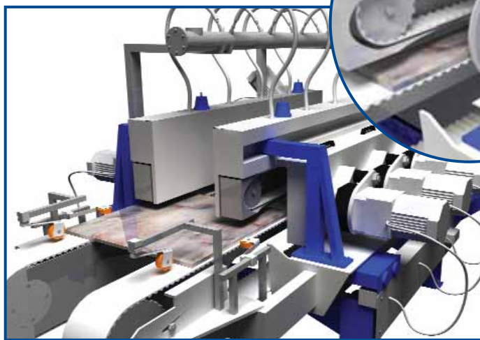
Tile squaring machine utilizes custom belts with precision ground thickness and width.
